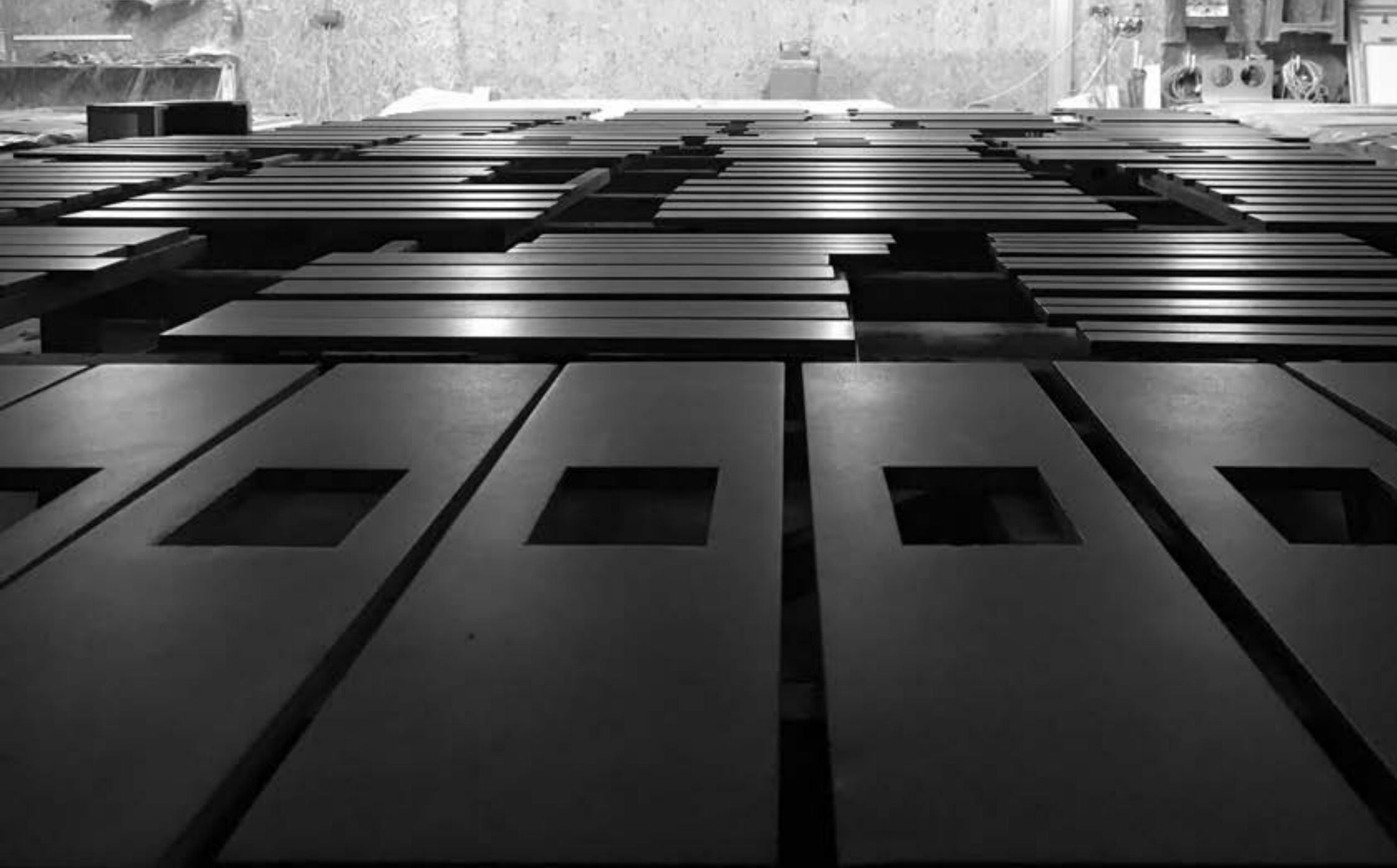
The Mayson Hotel concrete curing overnight in the workshop. We produced 99 sinks of 10 different sizes and in excess of 500 single
